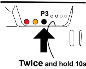
1- Press the push button **P3** **twice and hold** it down, the buzzer will make a beep each time and then sound quickly and intermittently.
