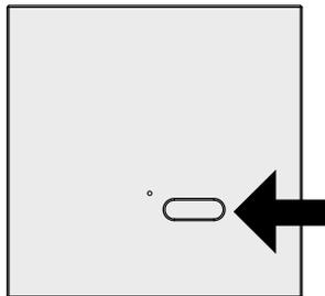
2- During the sound press the push-button which has to be deleted; the deletion is indicated by the continuously sound of the buzzer.
