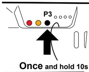
Push the push-button **P3 once and hold** it down for 10 seconds. The light turns on with a warm white colour and after 10 sec. it will flash once. The light will turn off at the release of the push button.
