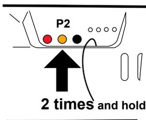
1- Press the push button **P2 two times and hold** it down, the buzzer will make a beep each time and then sound continuously.
