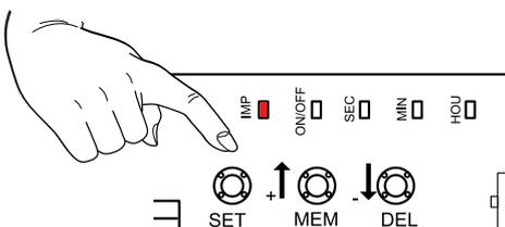
1- Press once and hold down the "SET" button until the led "IMP" lights up. Release the button and wait until the led goes out (the led will go out five seconds after the button is released and the settings will be saved automatically).
