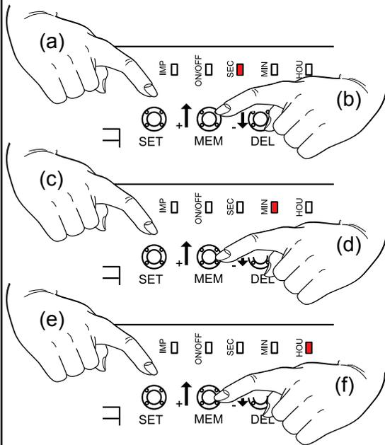
1- (a) To change the seconds, press the SET button three times and hold down until the SEC led lights up. (b) At this point we can change the seconds by increasing them using the MEM button or decreasing them using the DEL button. Each time we press the MEM or DEL button the led will go out and the value will be increased or decreased (e.g. 10 impulses correspond to 10 seconds).
