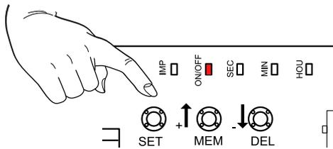
1- Press the "SET" button twice and hold down until the "ON-OFF" led lights up. Release the button and wait until the led goes out (the led will go out five seconds after the button is released and the settings will be saved automatically).
