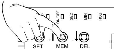
1- Press **twice** and hold down the push-button **MEM** of the receiver, the buzzer will make a beep each time and then sound continuously.
