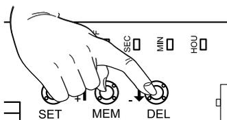
1- Press **once** and hold down the push-button **DEL** of the receiver, the buzzer will make a beep each time and then sound intermittently and slowly.
