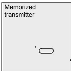
1- Press the button **P3** located inside the **already memorized transmitter**. The enabled receiver sound continuously.
