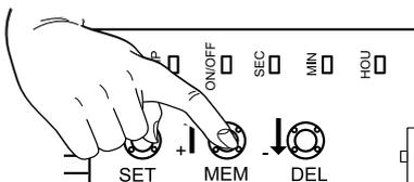
1- Press and hold down the push-button **MEM** of the receiver, the buzzer will make a beep each time and then sound continuously.
